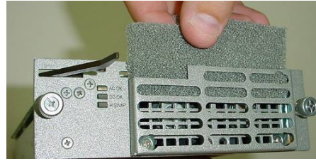
Figure 21 – Shelf Air filter and Power supply air filter extraction
