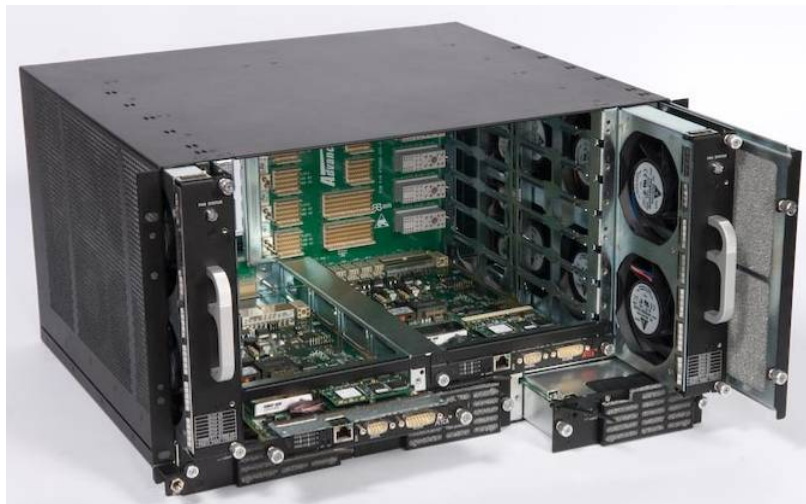
Figure 18 – Fan and Air filter trays
