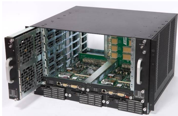
Figure 22 – Shelf fan tray extraction
