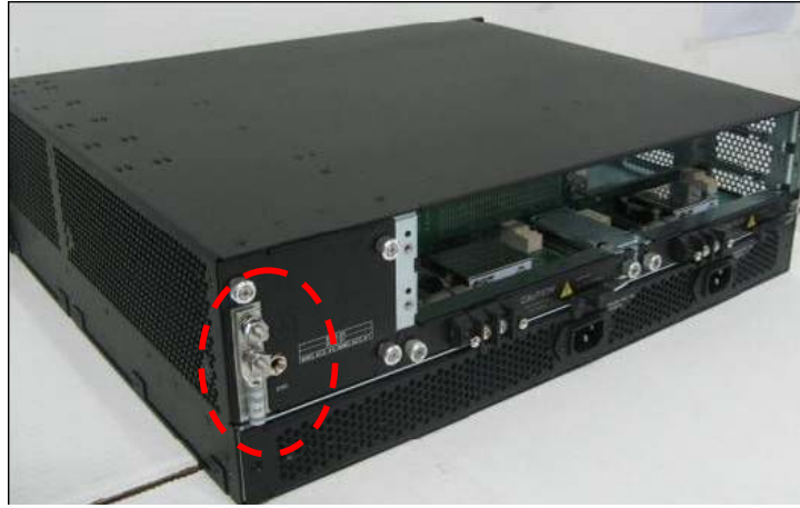
Figure 19 – Rear grounding screws
