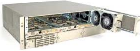
Figure 22 – Shelf Air filter and Power supply air filter extraction
