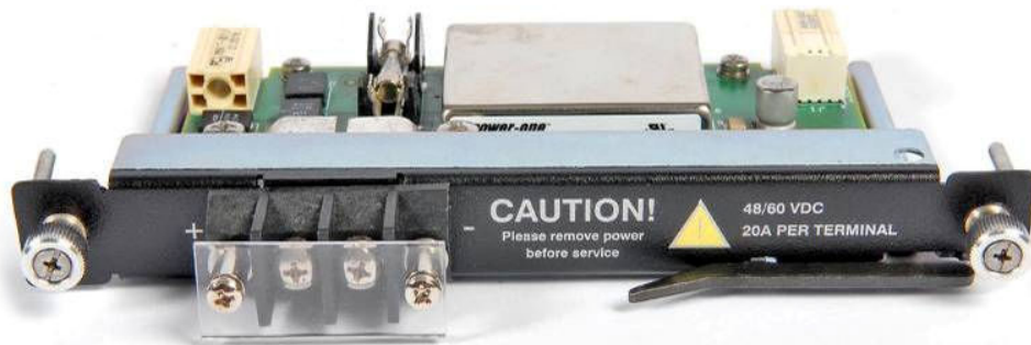
Figure 12 - ATCA DC PEM
