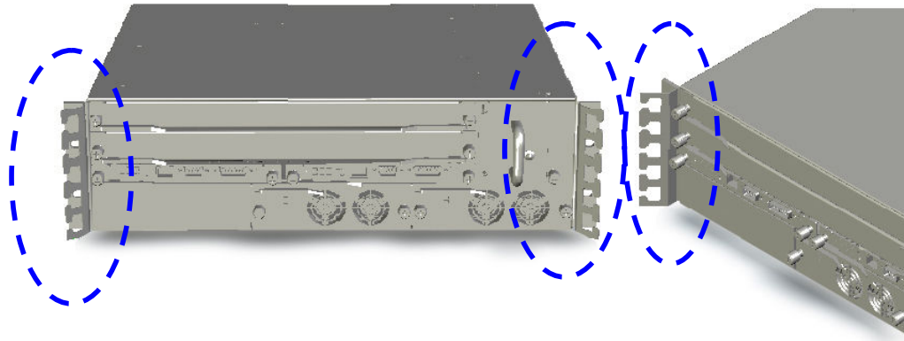
Figure 4 – Shelf Chassis with Cable Holders
