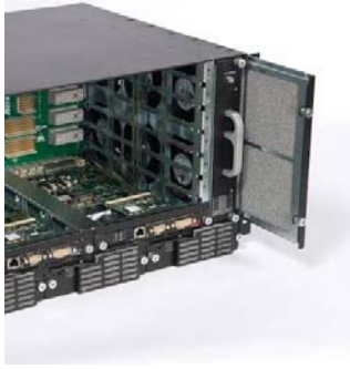
Figure 21 – Shelf Air filter and Power supply air filter extraction
